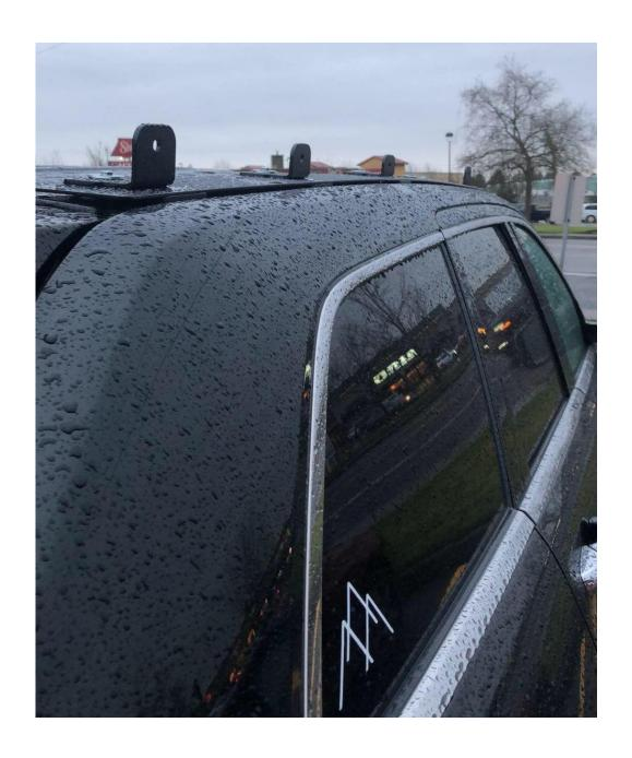
Step 4: Install Basket to Rails using 3/8's hardware (Bolt, lockwasher, flatwasher, through hole, with flat washer and nut on backside.
