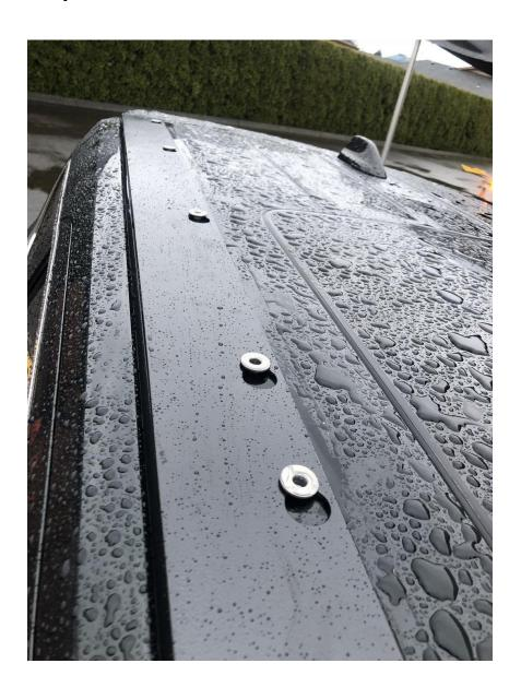
Step 3: Install washers and L Brackets, they are numbered, I, II, III, IIII— Install #1 to the front of the vehicle, working to the rear using #4. Tighen.
